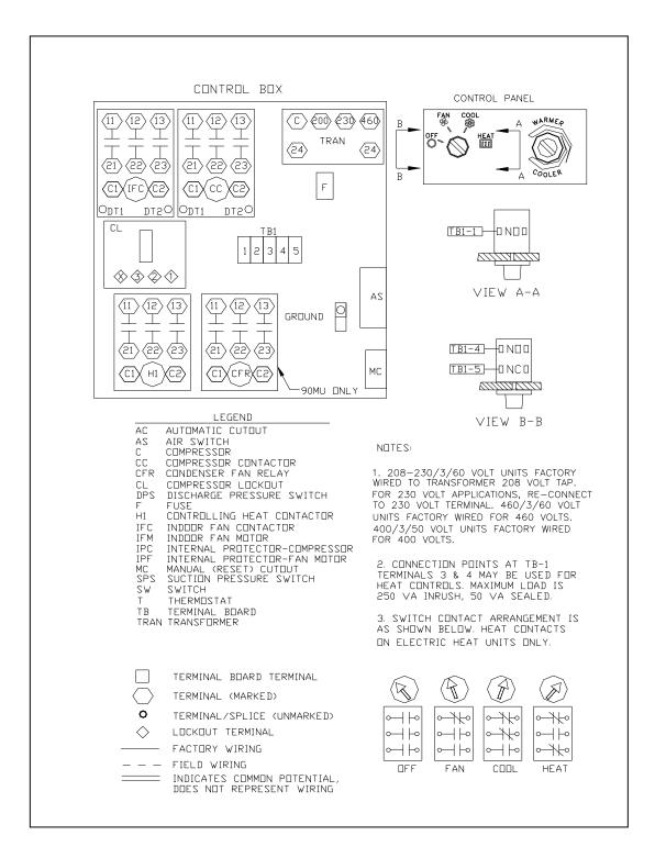
FIGURE 13 COMPONENT ARRANGEMENT - 90MA/MU\*04/\*06
